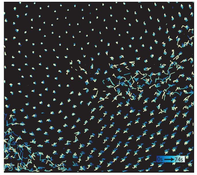
Glass under the transmission electron microscope: physicists observed the movements of individual atoms and can thus better understand the behavior of glass.
