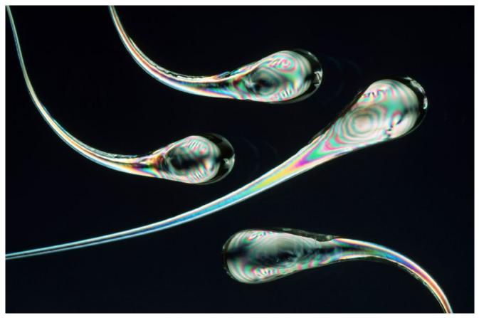
Glass suddenly cooled in water: The "Prince Rupert Drop" resists even hammer blows, but breaks immediately if his tail is damaged - due to internal stresses.
